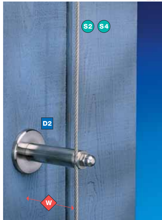
D2: Intermediate spacer (rope clamped) with maximum clamping force of 1 kN.
