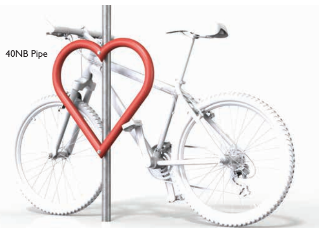
Units are designed to bolt-fix to existing 40NB or 50NB posts using M12 bolts & shear nuts
