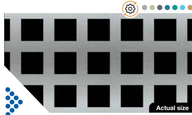
415 | Open area 44% 10.0mm square hole x 15.0mm straight pitch
