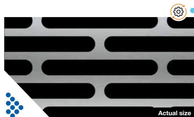
378A | Open area 60% Round slot 52.0mm x 7.0mm, staggered pitch
