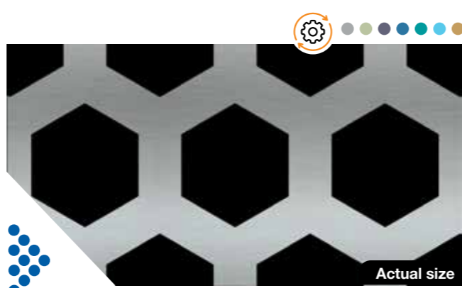
621 | Open area 51% 20.0mm hexagon hole x 28.0mm staggered pitch
