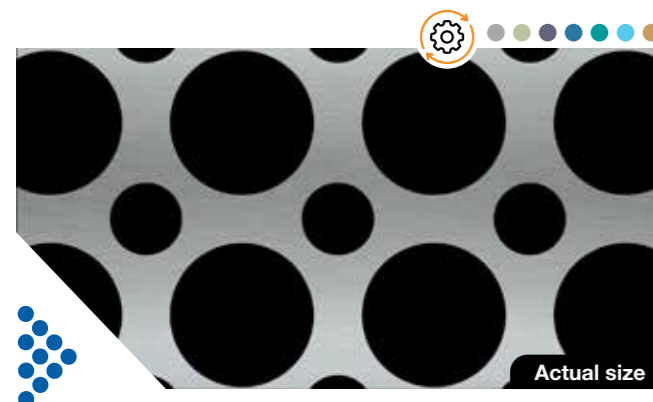
2459 | Open area 55% 19.0mm & 9.5mm diameter holes x 25.4mm straight pitch
