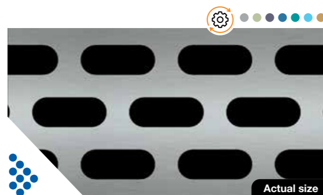
380 | Open area 40% Round slot 20.0mm x 8.0mm, staggered pitch
