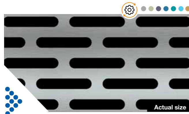
370 | Open area 40% Round slot 25.4mm x 4.8mm, staggered pitch
