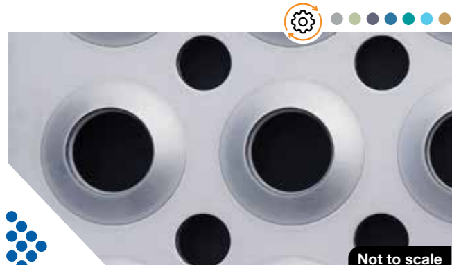
545 | Open area 23% 20.0mm diameter raised holes, 14.0mm diameter drain holes, 45.0mm straight pitch
