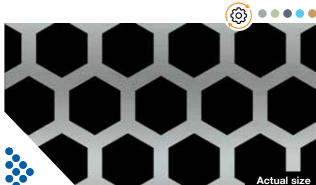
614 | Open area 60% 14.0mm hexagon hole x 18.0mm staggered pitch
