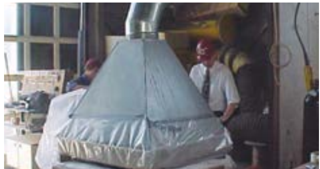
IFD air leakage testing at CSIRO.
