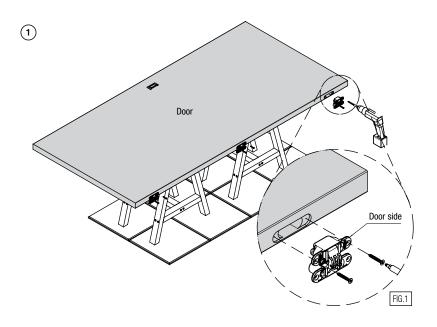
\*Set the hinges in the relative door leaf millings (fig.1) and fix them with the relative screws.
