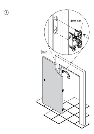
\*Fix the door leaf to the jamb and insert the hinges into the millings(see picture 2). Fix the hinges with the specific screws.
