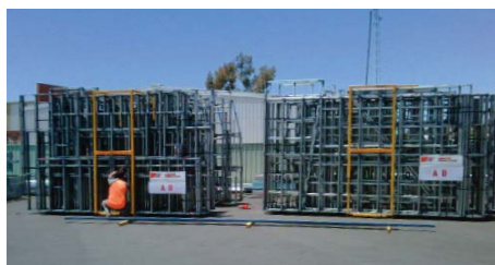
Pre-fabricated steel house frames ready for transport to the Outback for government housing program.
