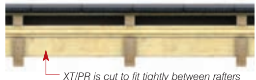
XT/PR is cut to fit tightly between rafters
