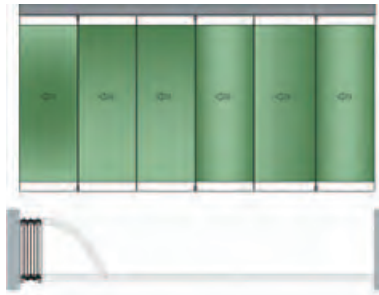
C. No access door (even panels, stack only).
