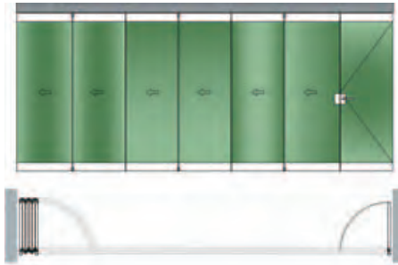
B. Access door opposite stack.
