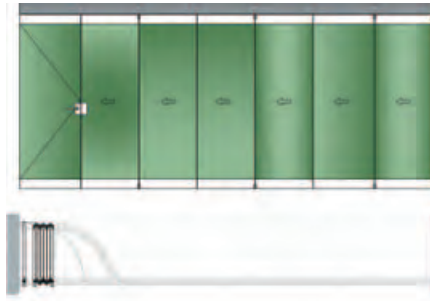
A. Access door at stack end.
