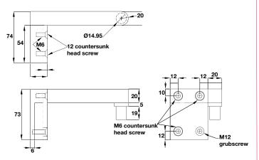
• Area of application: Pivot for Startec top patch fitting used on frameless glass pool gates
