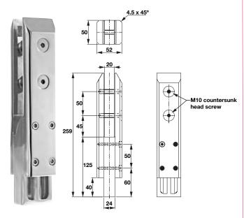
Frameless glass pool fencing Duplex 2205 grade stainless steel 10 mm, 12 mm and 15 mm • Area of application: • Material: • For glass thickness: • Installation: Clamp fixing with hexagon bolt
