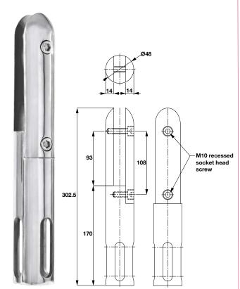
• Area of application: Frameless glass pool fencing Duplex 2205 grade stainless steel • Material: For glass thickness:Installation: 10 mm, 12 mm and 15 mm Clamp fixing with hexagon bolt
