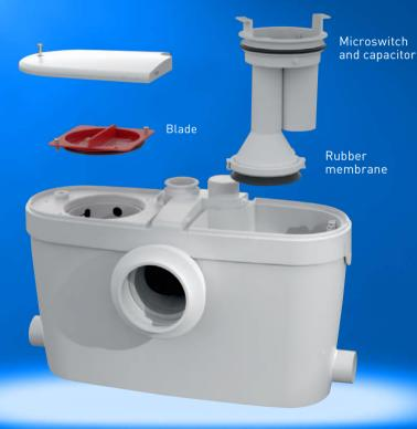
Pumping distance of up to 5m vertically and 100m horizontally Three water inlets to accommodate a toilet, sink and shower
