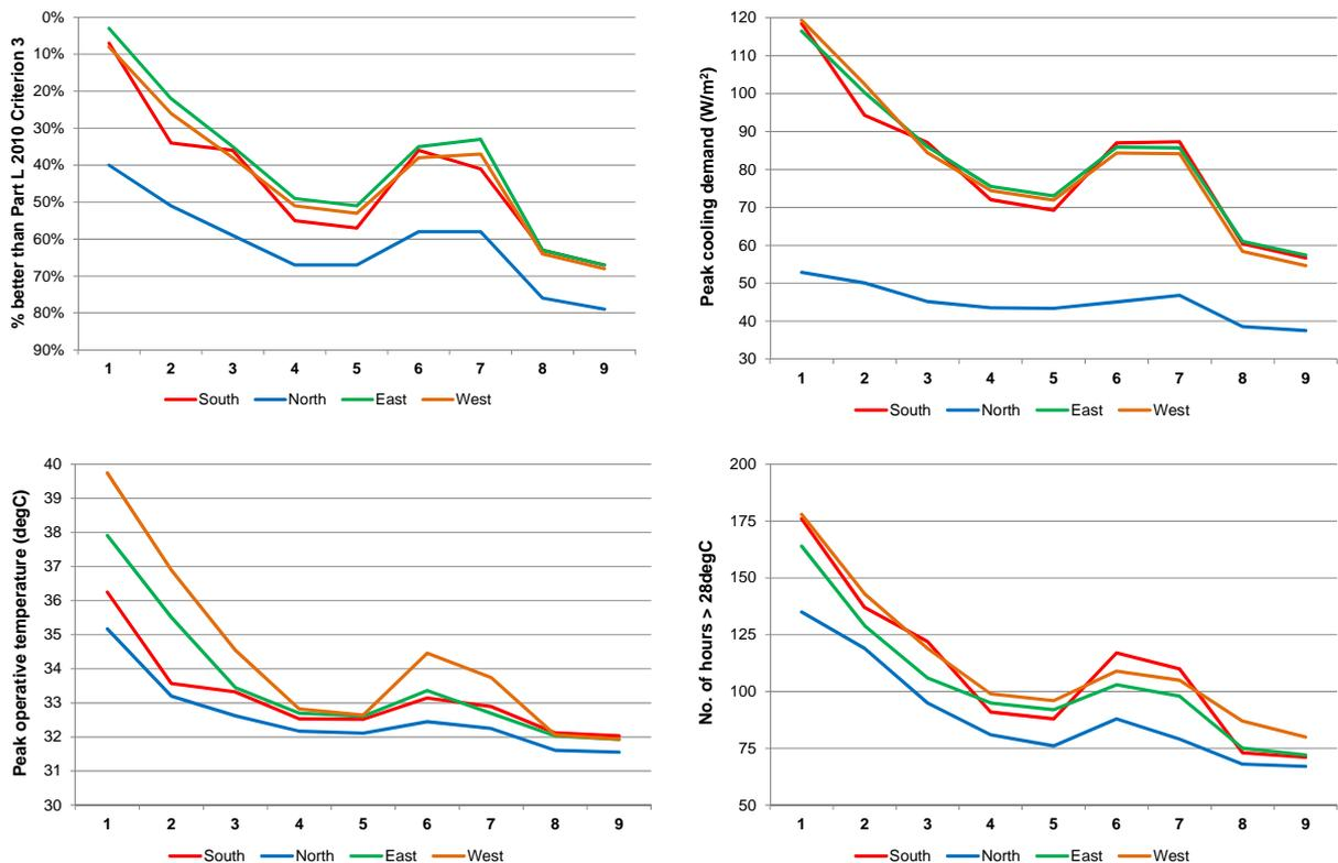
**Fig 3** Thermal comfort indicators for different façade options and orientations
