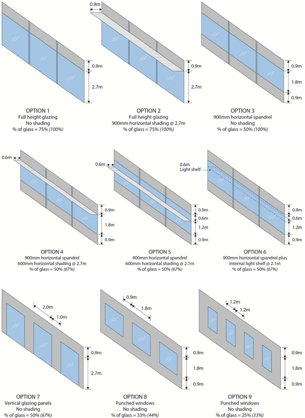
The percentage of glass is based on the floor to floor façade area. The percentage of glass in brackets is based on the floor to ceiling façade area (i.e. the occupied zone).
