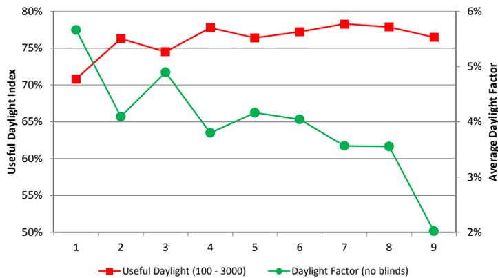
Fig 4 Daylight factor (DF) versus Useful Daylight (UDI) in 6 m deep perimeter zone for nine façade options
