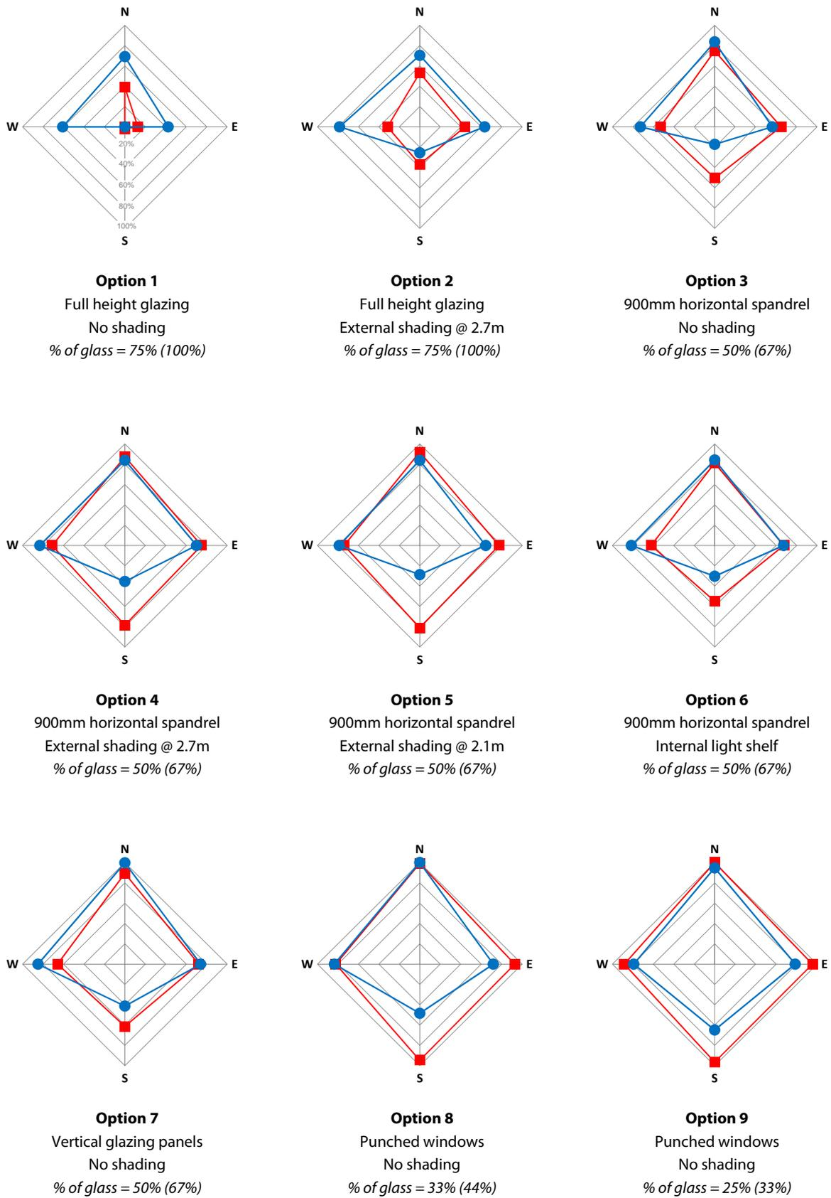
Fig 6 Thermal comfort and daylight comparative scores for different façade options
