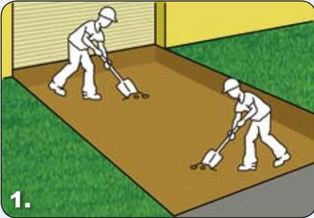
Excavate the area out at approx. 230mm of depth. Base of excavation should be flat and relatively level.
