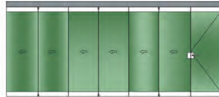
B. Access door opposite stack.
