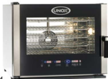
XVC 304 Combi-oven 5 GN 1/1; spacing 67 mm 240V/415V3~; 5.3/3.2 kW Max. temperature 260°C 750mmW x 728D x 625H; 55 kg
