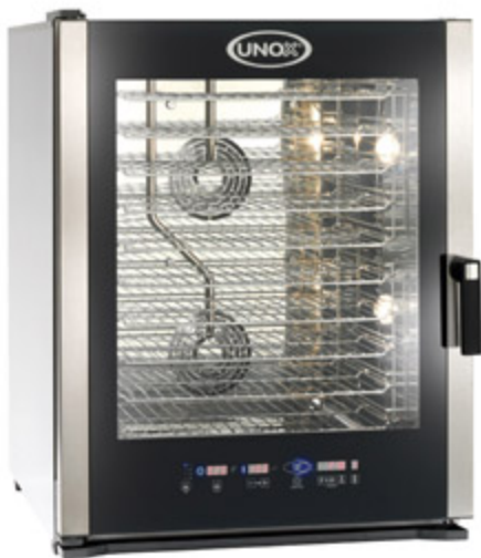
XVC 704 Combi-oven 10 GN 1/1; spacing 67 mm 415V3~; 10.5 kW Max. temperature 260°C 750mmW x 728D x 960H; 77 kg
