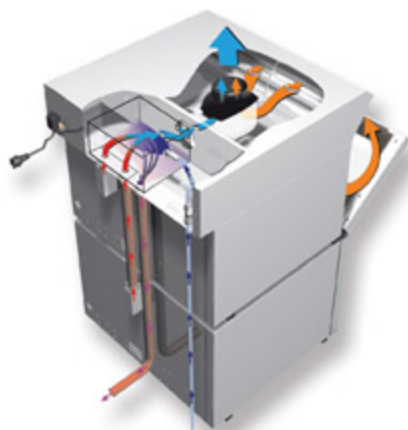
Hood with 2-speed fan & steam condenser scrubs & cleans exhaust fumes option XC 314 stand alone fume condenser option XC 114
