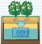
Passive irrigation water source using Flo-Tank®
