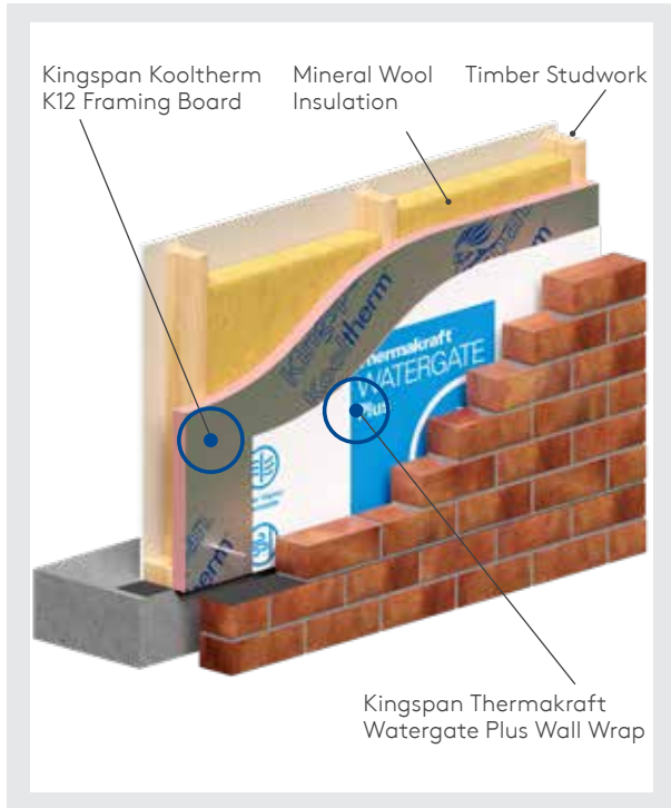
Externally Lined Continuous Insulation for Timber Frame
