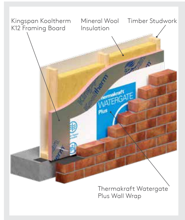
Figure 4. Externally Lined Insulation
